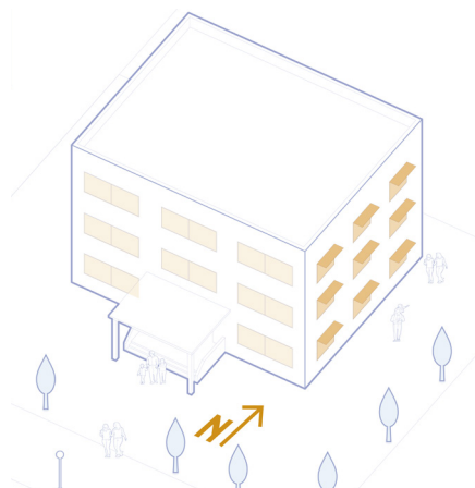
Smaller windows to the east, west and south. Window shading to mitigate sun impact. [ Guideline 3.5.7 (1) ]
