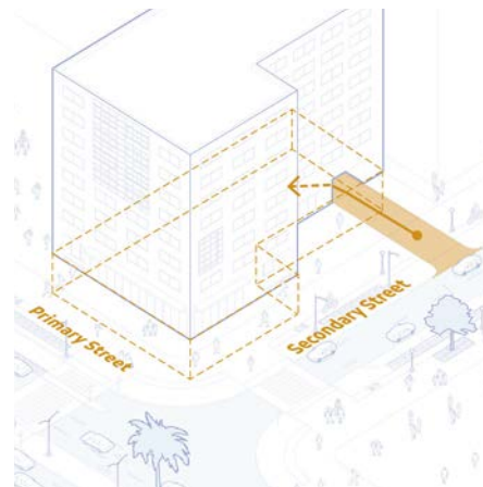
Underground parking encouraged, with parking access not from the primary street. [ Guideline 3.4.8 (2) ]
