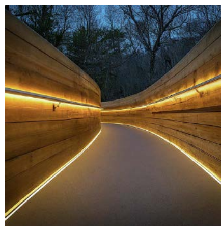
Steps, ramps, and edges of pedestrian pathways should be illuminated for safety. [ Guideline 7.11.12 ]
