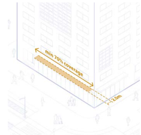
Building frontage to have at least 2.0 meters of shaded clearway min 70%. [ Guideline 3.4.7 (4) ]
